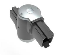
**Additional information:** Use Intermediate Joint to join two horizontal tubes together for a longer run. The arm can be rotated or turned 300 degrees. Includes safety stop and maintenance-free bearing. RAL 9005 black finish. Die-cast aluminum construction. Includes two removable cable access covers, installation instructions, gaskets and tube setscrews. Use of the Intermediate Joint reduces the system load capacity to 179 lb. (81.2 kg) at 3.3 ft. (1 m).
